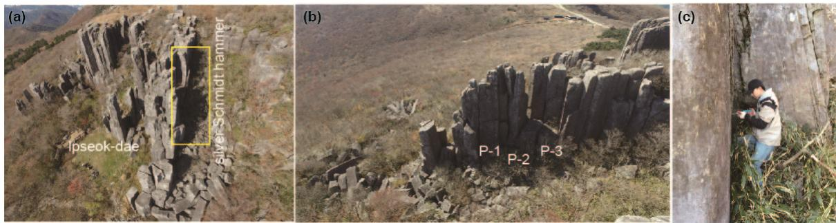
Fig. 9. Silver Schmidt hammer test at the Ipseok-dae, (a) aerial photograph, (b) measuring place, (c) field measurements.
